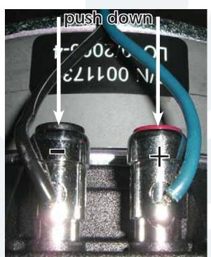
The positive (blue and black) and negative (solid black) cables are still attached to the woofer terminals. Remove the cables from their terminals simply by pushing down on the terminal and pulling out the cable.
